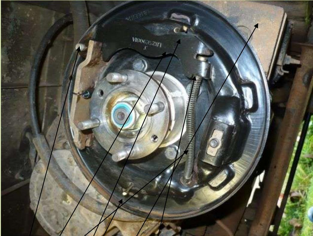
Handbrake cable and spring
