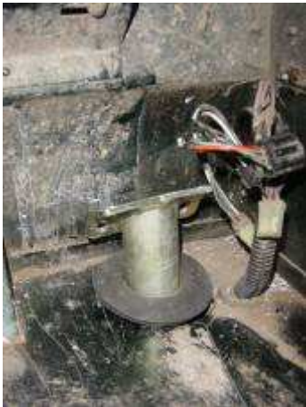
View looking up inside the rear wheel arch. Rubber grommit can be viewed through the hole.
