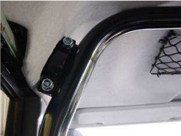
View of the internal B-pillar hoop bolted through to the external roll cage bar.
