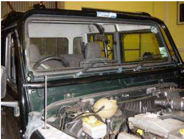
With the two front internal struts in position and fixed to the chassis, fit the front windscreen hoop and lower windscreen bar. Insert the bolts and loosely fix their nuts keeping the front hoop in position.
