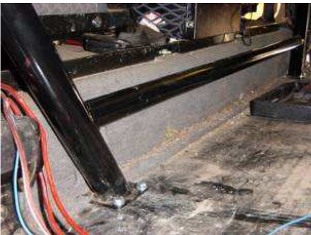
B-pillar hoop bolted in and complete.
